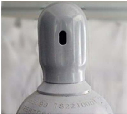
Figure 4 Cylinder with shroud for valve protection
