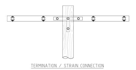
Figure 2-2: Typical arrangement at termination/strain locations
