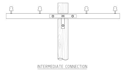
Figure 2-1: Typical arrangement at intermediate locations
