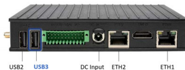
Figure 9: Horizon Power's SGD hardware and port overview 1
