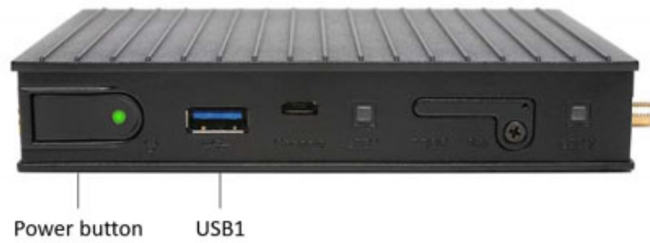
Figure 10: Horizon Power’s SGD hardware and port overview 2
