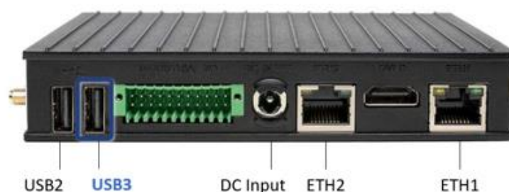
Figure 2: Horizon Power's SGD hardware and port overview 1
