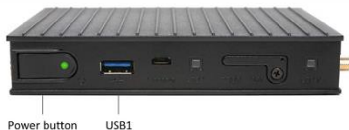
Figure 3: Horizon Power's SGD hardware and port overview 2
